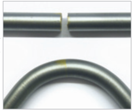
Figure 7 | Steel rods brazed at about 830 °C. Top: with silver-free brass brazing alloy *) , the brazed joint is not ductile; Below: with BrazeTec 1204, the brazed joint is ductile.
