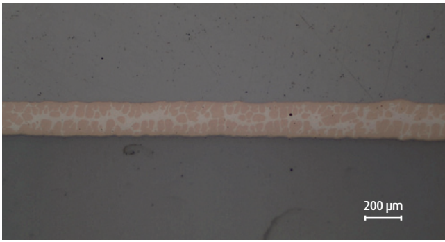
Figure 26 | Brazing BrazeTec 49/Cu at 1,100 °C in a 180-second cycle
