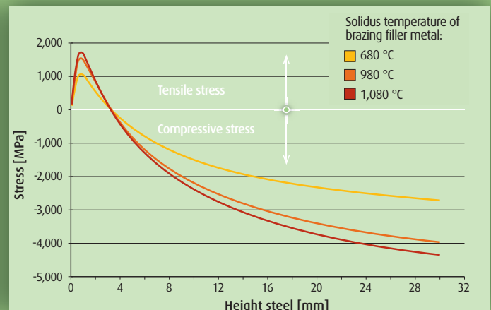
Figure 9 | Stress state in a cemented carbide surface 1 mm thick connected to steel layers of varying thicknesses
